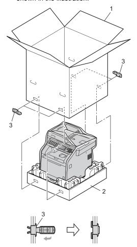
Put the two Styrofoam pieces (1) into the carton matching the right of the machine to the "RIGHT" mark on one of the Styrofoam pieces, and the left of the machine to the "LEFT" mark on the other Styrofoam piece. Put the AC power cord and printed materials in the original carton as shown in the illustration.
